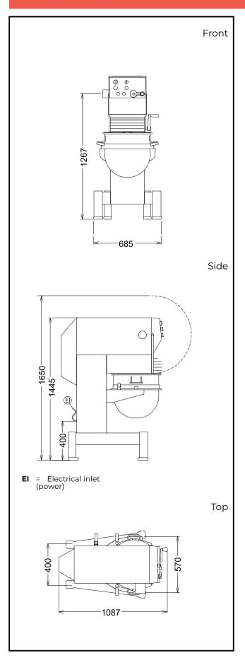
Electric 220-240/380-415 V/3 ph/50 Supply voltage: Electrical power max: 1.54 kW **Total Watts:** 1.54 kW Capacity: ISO 9001; ISO 14001 kg/ Performance (up to): Cycle Capacity: 60 litres Key Information: External dimensions, 685 mm Width: External dimensions, 1087 mm Depth: External dimensions, Height: 1445 mm **Shipping weight:** 337 kg
